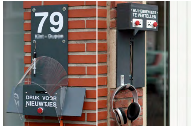
Figure 3: Left: Readl with integrated house number. Engraved message reads, “ Push for news ”. Right: Listen with headphone. Engraving reads, “ We have something to say ”.
